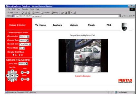
Using the server-push viewer, some functions such as 'Progressive Mode' image transmission, 'Image Quality' control, and 'Quality Box' creation menus out of image control and 'Preset', and 'Focus Sensitivity' control out of PTZ control are not supported. Other functions are the same as that of the default viewer.
